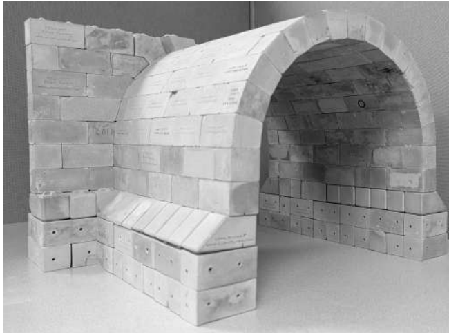
Arch-Lock™ structure constructed with model blocks
